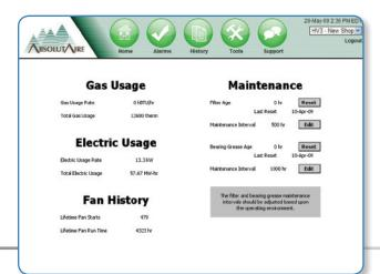
**Tools.** Maintenance intervals can be customized using the edit functions. When the filter age or bearing grease age exceeds its pre-set service interval, an alarm is activated.
