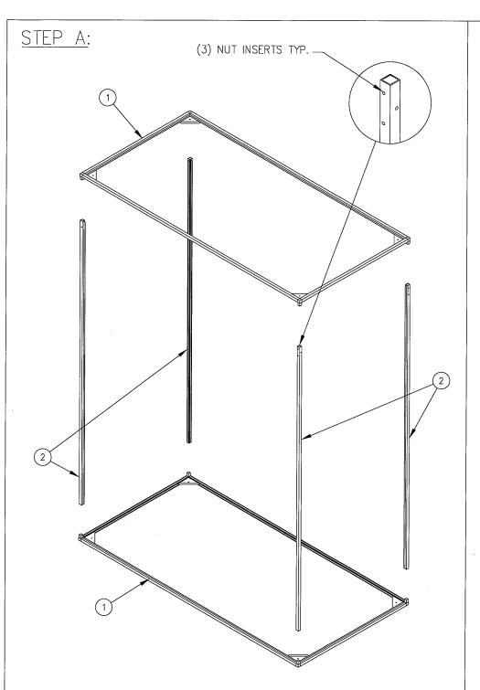
Assemble 1-1/2" tube frame using items 1 & 2. Item 2 has (3) 1/4-20 nut inserts in one end only. Orient item 2 the same direction for all (4) pieces. See detail above.
