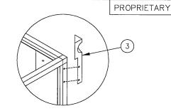
Attach lifting lugs (item 3) using (3) - 1/4-20 bolts. (4) lifting lugs total, (1) per corner.
