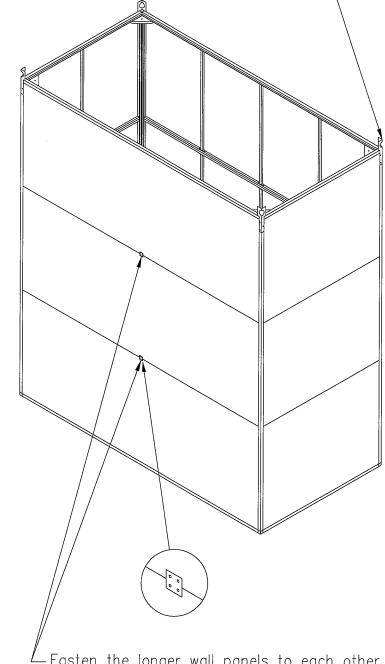
Fasten the longer wall panels to each other using item 4. See diagram above.
