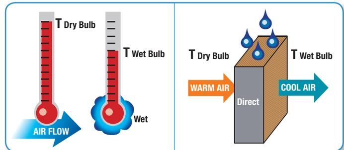
An evaporative cooler with 88% saturation efficiency will cool the air by 88% of the difference between the two air temperatures. For example, if the dry bulb temperature is 90°F and the wet bulb temperature is 70°F, this evaporative cooler can cool the air to about 72.4°F (90°-70° = 20° X 0.88 = 17.6° and 90°-17.6° = 72.4°)
