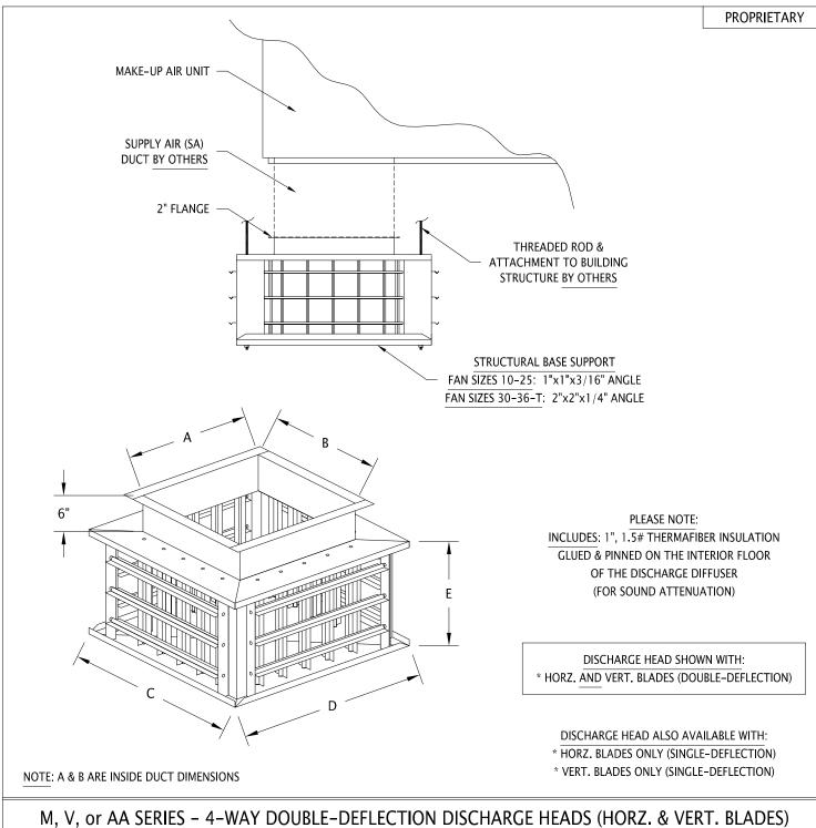
SIZE OF DISCHARGE HEAD WILL VARY DEPENDING ON BLOWER, UNIT MODEL/SIZE, VIBRATION ISOLATION (IF APPLICABLE), ETC. CONSULT FACTORY TO DETERMINE WHICH DISCHARGE HEAD WILL BE USED FOR YOUR SPECIFIC APPLICATION.
