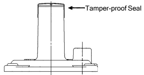
Permanent pressure sensitive backed paper. Attempted removal of these seals will destroy the face stock, leave adhesive residue on surface beneath, thus tampering can be easily detected. Available for all threaded models. Outlet pressure printed on seal.
