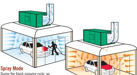
During the finish spraying cycle, an AbsolutAire direct-fired system typically provides 100% outside air (OA) that is tempered to between 60° and 90°F and supplied in constant high volumes for maximum booth ventilation.
