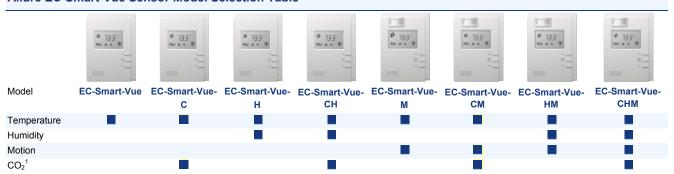
The Allure EC-Smart-Vue sensor CO<sub>2</sub> models must be used in spaces that are periodically unoccupied (e.g. during evening or nighttime hours). A
