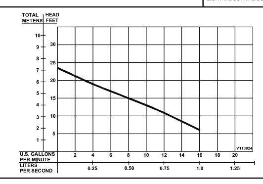
Testing is performed with water specific gravity of 1.0 @ 68°F (20°C), other fluids may vary performance
