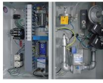
Reliability and safety are ensured with advanced gas-manifold controls, electronic ignition, flame rod burner supervision, and diagnostic circuit check lights.
