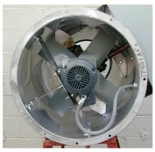
High-volume airflow with consistent velocity is provided by a large, directdrive axial fan on the inlet end.
