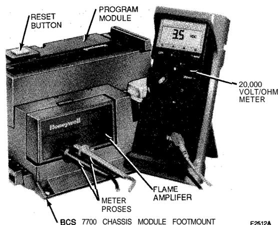
**Fig. 9c—Measuring flame signal voltage of 7900 SERIES controls.**
